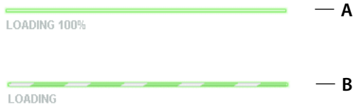
Top. Determinate ProgressBar control Bottom. Indeterminate ProgressBar control
